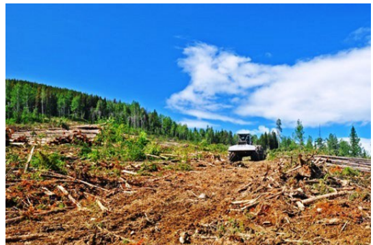
Figure 3: Proper equipment, such as this wide-tired skidder, and proper techniques to reduce impacts to soil
